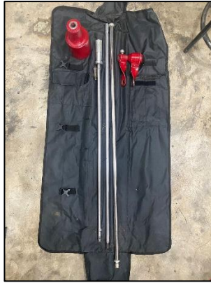
Gambar 6. 1 Dynamic Cone Penetrometer
